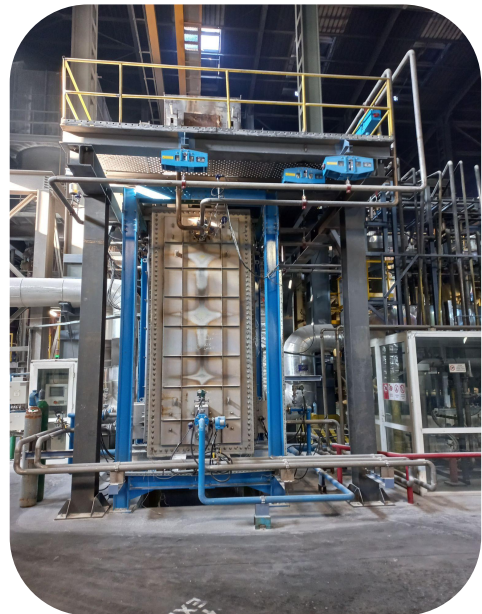
By-pass flue gas channel on the left side and on the right side the radiative heat-exchanger
